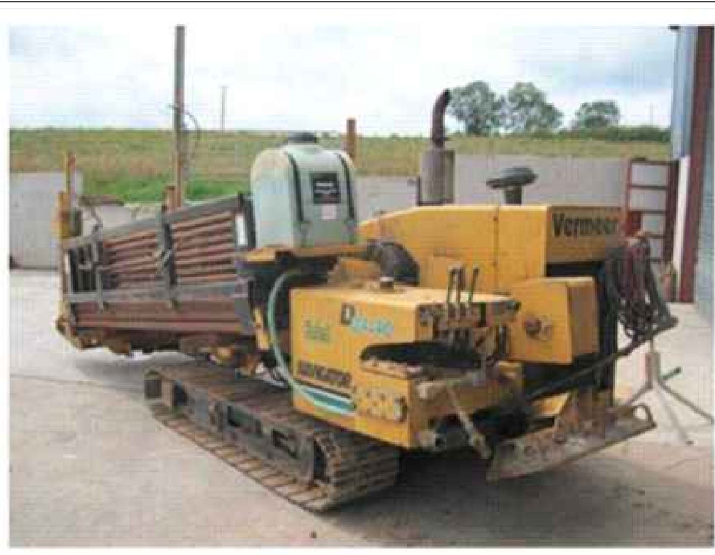
Image 2 | Typical Directional Drilling Rig
